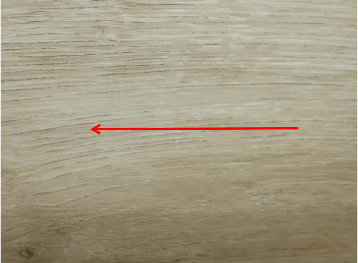
Figure 1: Urban Naturals Rustic embossing vinyl plank Arrow indicates direction of testing
