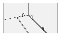
4 **Install the second row:** Use the off-cut from the first row to start the second row. It must be >300mm, and not closer than 300mm from the end join in the previous row.
