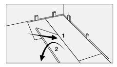
Check to be certain all planks are fully engaged; if slight gapping is noticed or the planks will not lay flat, simply disengage the long/top side join and then carefully slide the short/end join apart. Do not pull up on this join as it will damage the locking mechanism. Reinstall the plank.
