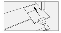
Internal expansion gaps are required at doorways/thresholds and rooms exceeding 30mx15m.
