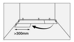
**Tap Fold-down (Unipush®):** Long side first, then fold down and gently tap the end-join ensuring it is properly aligned.
