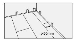
10. Remove spacers/wedges from around the room and install skirting boards and/or Godfrey Hirst scotia and/or finishing trims (in accordance with Godfrey Hirst accessories installation guidelines). Never fix any trims directly to the floor and ensure fixing does not compromise expansion gaps. Silicone or caulking compound is not recommended.
