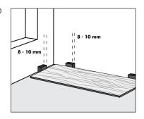
Continue the first row ensuring each board positively locks on the end joints. Insert the board on an angle and lower it down to engage the lock.
