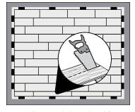
scribe and cut this final row, while retaining the 10mm expansion gap.
