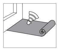
all joints are overlapped 300mm and taped using a vapour-tight tape.
