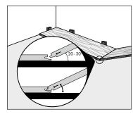
At the end of the run measure and cut the board to the required length, ensuring you leave 8-10mm for the spacer.
