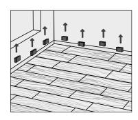
Reinstall the skirting boards or finish the perimeter of the floor with a complementing trim, such as scotia.
