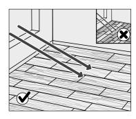
The floor should never be fixed or glued at any point.
