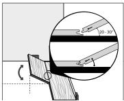
The first board of the second row locks into place by inserting the long side on an angle, then pushing down to engage.
